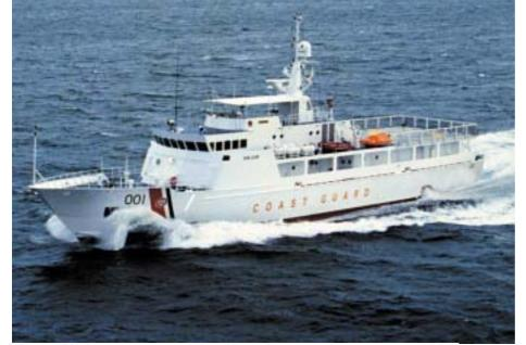
Communications to Det Norske Veritas rules, and has a steel hull and aluminium superstructure.
